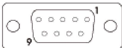
To operate in RS485 pins 4-3 and 8-7 must be connected externally.
