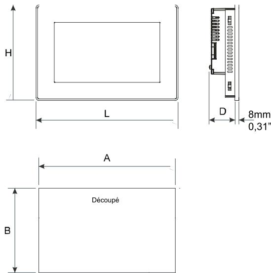
*Fig. 2 Dimensions BTM-T15-PLUS*
